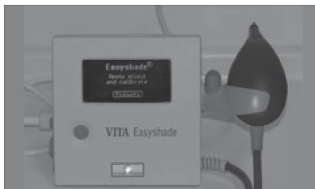
Fig. 3. Clinical spectrophotometer VITA Easyshade.
