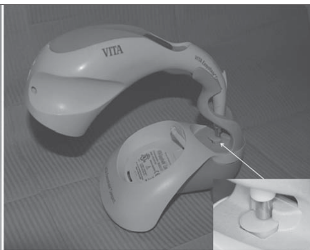
Fig. 2. The experimental setup with the Clinical Spectrophotometer VITA Easyshade Compact.
