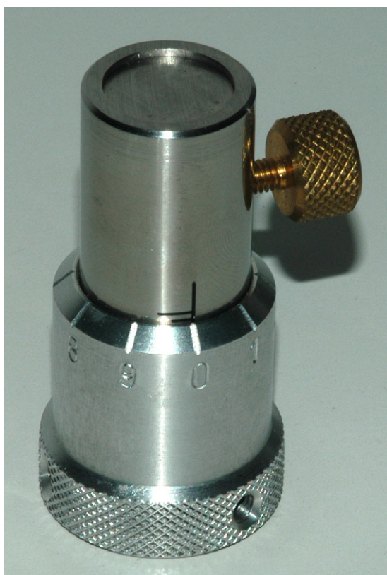
Fig. 1 – Calibrated mold used for manufacturing specimens in controlled thickness.
