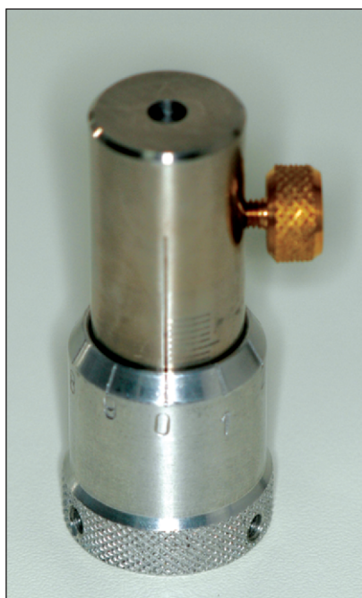
Figure 2: Cylindrical stainless steel mold used for specimen manufacturing.
