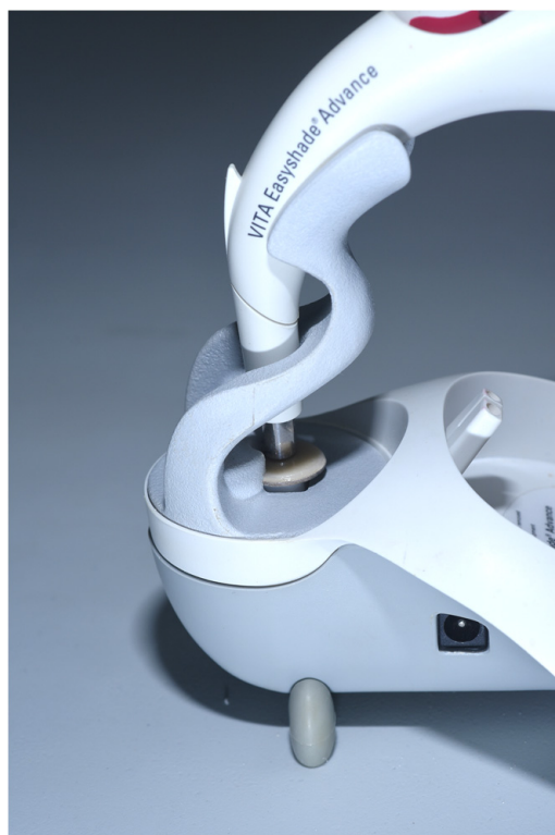
Figure 2. The clinical spectrophotometer VITA Easyshade fixed on a stand for color measurement.
